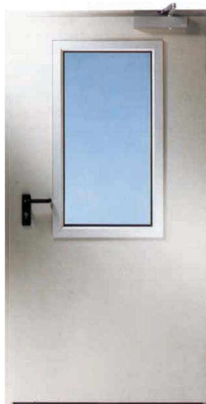
Fire-resistant door T30-1 Novoferm N2/50 with 460 x 910 mm glazing, door closer as standard; illustration with aluminium cover strip (special equipment, extra charge).
